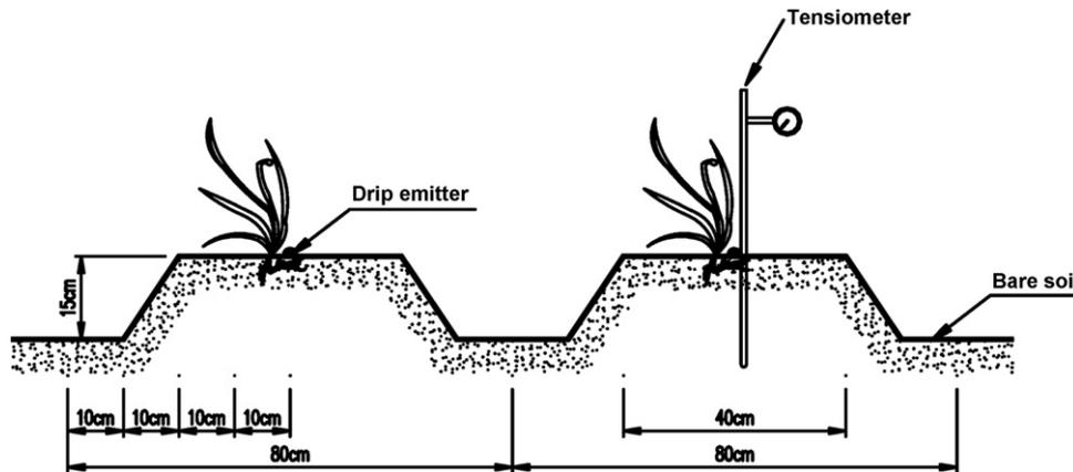
Fig. 1. The schematic diagram of ridging.
